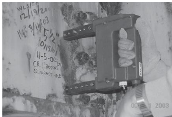
Magnetic particle testing—Placement of magnetic field.
